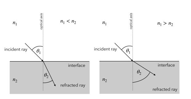
light is refracted at interfaces
